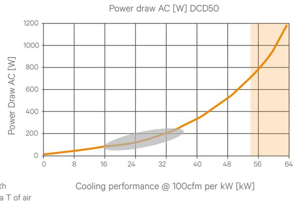
**Error mode** -> with 3 fans higher delta T of air
